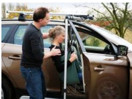
**Hoist** - are usually fitted to the car to help lift someone in and out, but necessity much time than other devices. Hoists may not be suitable for all children. A child that is prone to spasms will be difficult to hoist safely, and the sling can cause damage to the skin through shearing.
