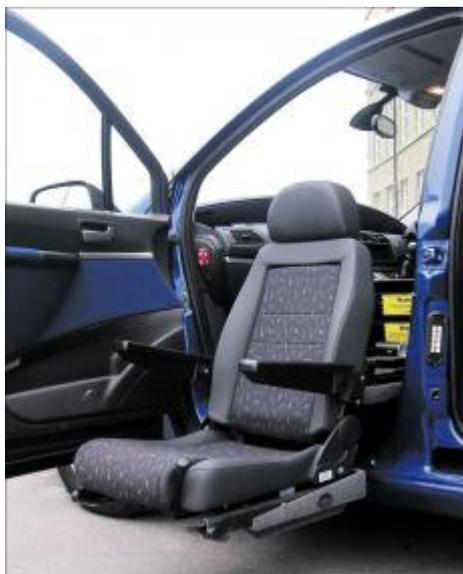
**Swivel device/seat** - A transfer device that turns or swivels provides support for an individual between seated positions and also provides ergonomically correct positioning for the personal assistant. This tool reduces the risk of falling or accidents and can be easily pushed out of the way when not in use. It should only be utilized with those who can stand with support and can bear their own weight, and is designed to aid in transfers between a wheelchair and a bed or toilet.
